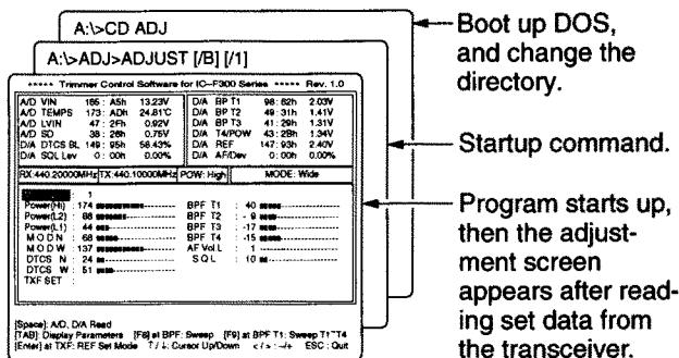
**NOTE:** When the EEPROM (FRONT unit; IC3) is replaced or the transceiver displays an error message and beeps, the following operation is necessary before starting the ADJUSTMENT.
