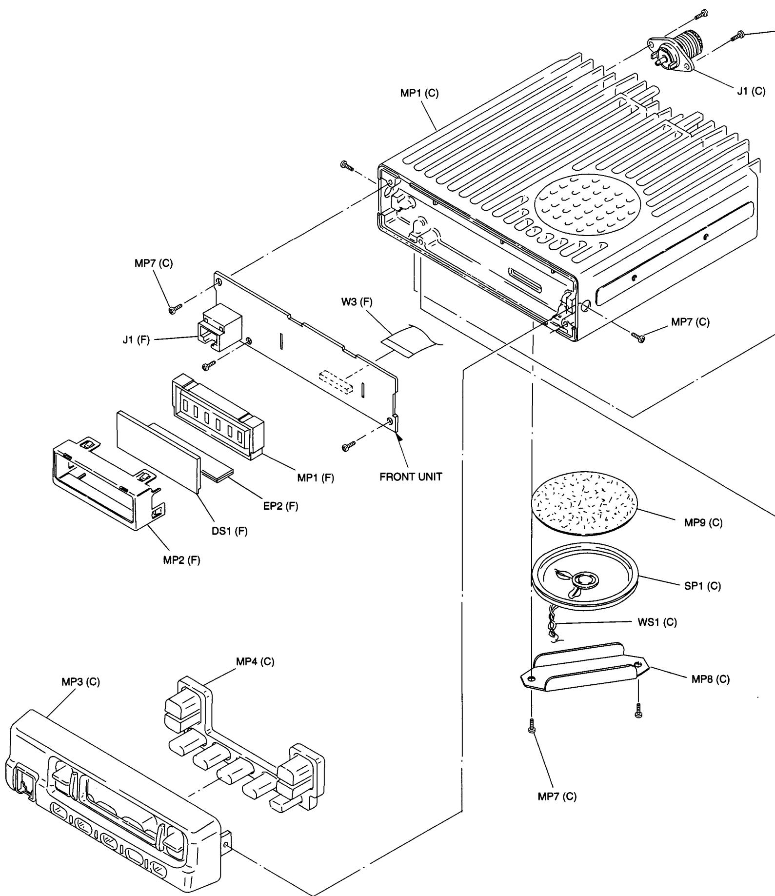
**Unit abbreviations** (F): FRONT UNIT (M): MAIN UNIT (C): CHASSIS PARTS
